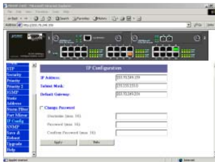
Figure 3-16 The IP Config page
